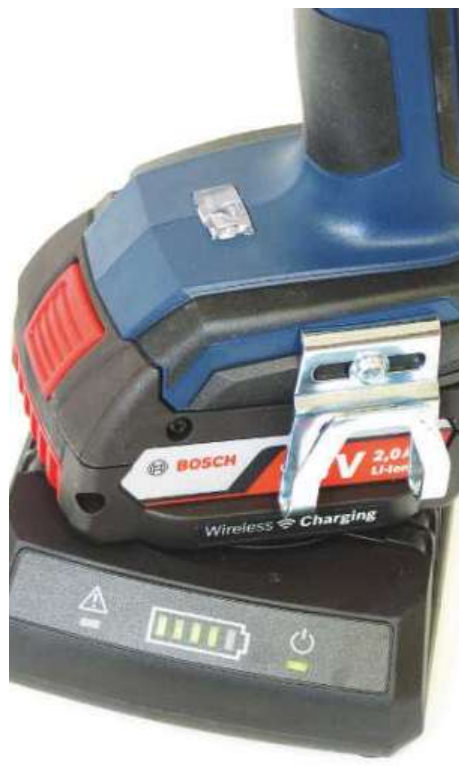
▲ A green light shows that the battery is in the charging zone, however haphazard its placement
